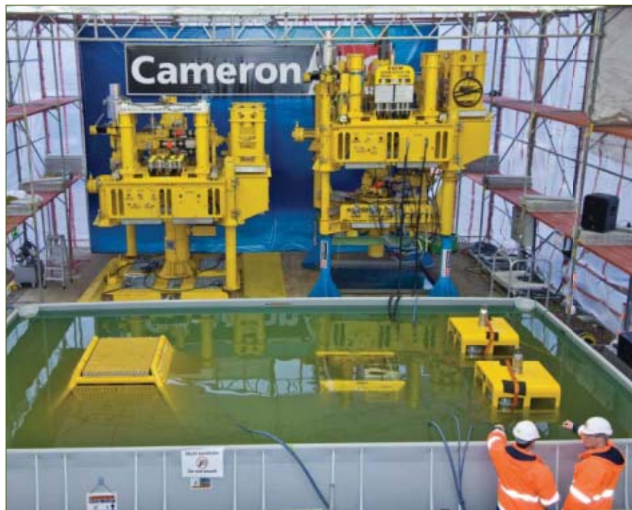
Cameron's site integration test (SIT) program included a water basin filled with seawater for simulating the electrical current return path (Fig. 6).
